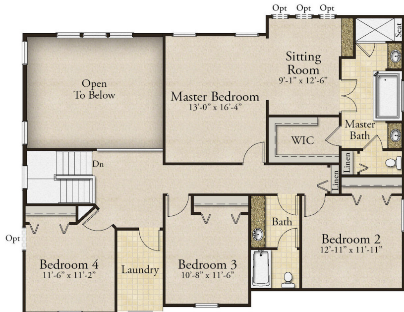
Opt. Second Floor Layout with Executive Master Suite (Shown with Opt. Dry Bar)
